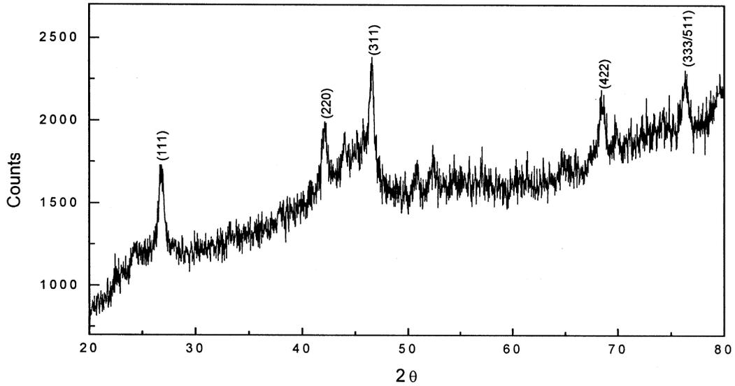
Fig. 1—Powder X-ray diffraction pattern of the nanocrystalline NiFe<sub>2</sub>O<sub>4</sub> of an average particle size 25 nm
