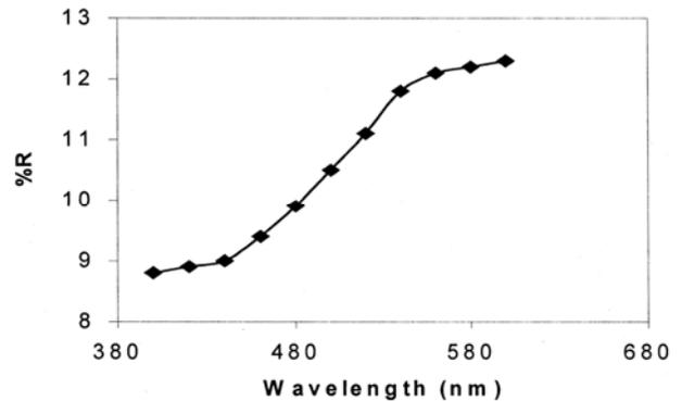
Fig. 2—Reflection spectra of NiFe<sub>2</sub>O<sub>4</sub> pellet
