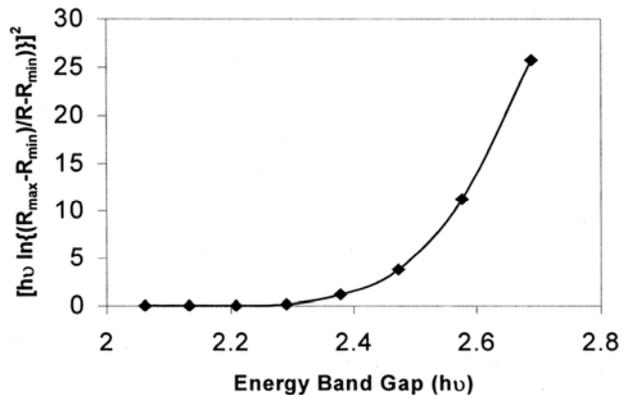
Fig. 3—Band gap determination of NiFe<sub>2</sub>O<sub>4</sub> pellet. The extrapolation of straight line to  $(h\nu)$  axis gives the value of energy band gap. The estimated optical band gap is 2.5 eV
