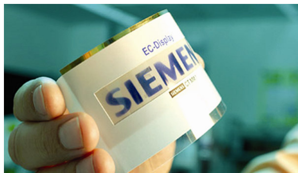
Fig. 3—A flexible electrochromic display, as developed by Siemens
