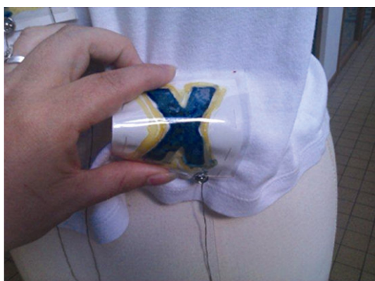
Fig. 8— The flexible electrochromic device (a) before and (b) after an electrical current has been applied
