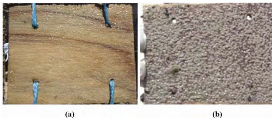
Fig. 8—Variations in fouling pattern observed on the test panels between two successive weeks. (a) From 8 th - 15 th June, 2006, (b) From 15 th - 22 nd June, 2006
