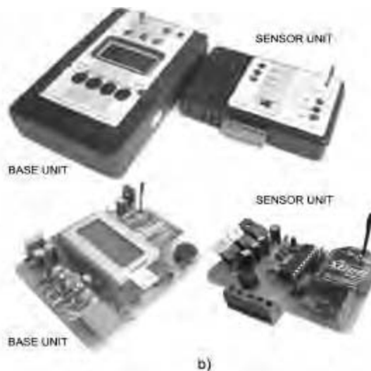
Fig. 2—Wireless filter monitoring system (WFMS): a) Block diagram; and b) Prototype
