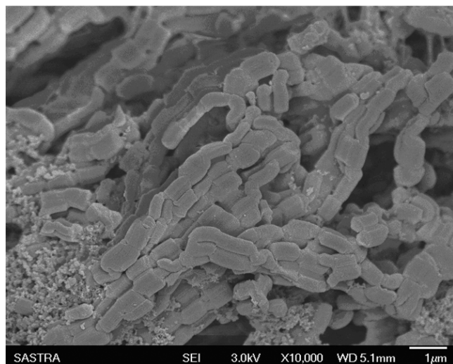
Fig. 2—SEM image of SBA-15
