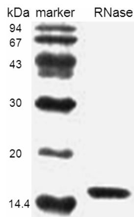
Fig. 2—SDS-PAGE of purified RNase (fraction SU2) [Lane 1: Molecular weight markers, from top downwards, phosphorylase b (94 kDa), bovine serum albumin (67 kDa), ovalbumin (43 kDa), carbonic anhydrase (30 kDa), soybean trypsin inhibitor (20 kDa) and lactalbumin (14.4 kDa); and lane 2, purified RNase]
