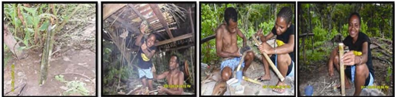
3c. Bamboo processing: Cut bamboo, clean the leaves and twigs that are not used then cut in the sections to be used. Hang on the furnace until it dry and become yellowish. After that, Cut the bamboo with the size desired.
