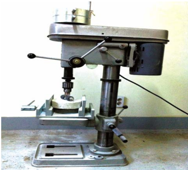
Fig. 4 – Abrasion test set-up
