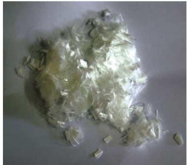
Fig. 2 – Shape of nylon fibers
