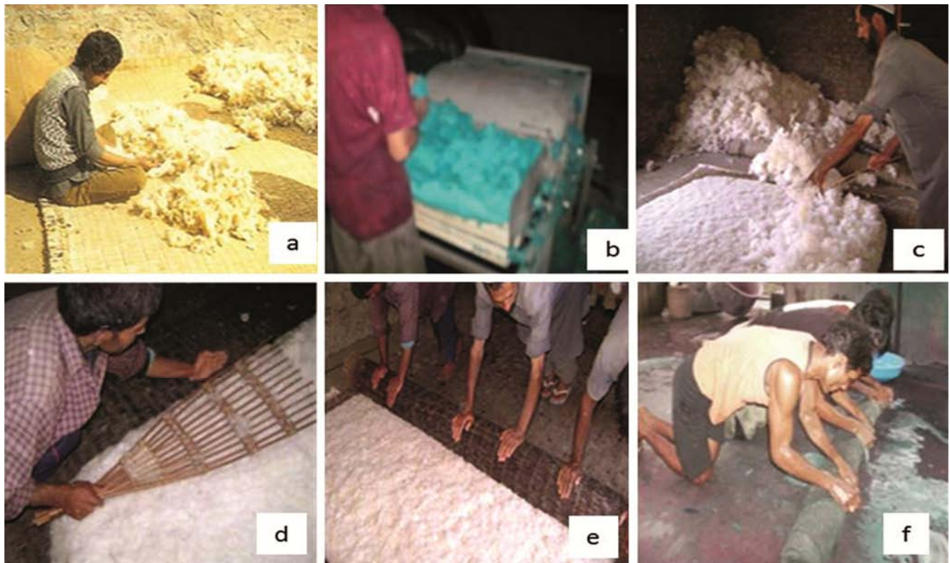
Fig. 1—Process of namda manufacturing, a) manual sorting ( pinai ) of wool, b) mechanized carding machine, c) cleaning and laying of wool, d) flattening of the layered wool with a punjah , e) rolling of moistened namda on a wooden stick, f) traditional ghutai of namda
