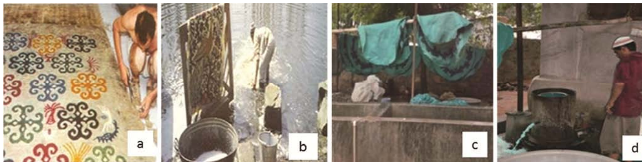
Fig. 3—Finishing of namda , a) cutting the edges for finishing with a scissor ( kenchi ), b) washing of namda in the river Banaas , c) sun drying of washed namda , d) mechanized drying of namda in a boiler.
