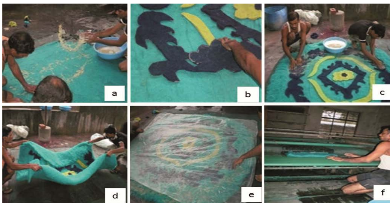
Fig. 2—Milling and design placement on namda . a) Spraying of soap water, b) Laying the prepared designs, c) Sancha bhara ' or final design allocation on namda , d) Laying of designed namda for milling, e) Covering of namda with a plastic sheet and then rerolled for milling, f) mechanized milling of namda
