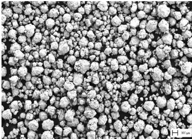
Fig. 9—Structure of powder \text{Cu}_{50}\text{Ti}_{50} after 7 h of mechanical alloying, SEM images at 100 magnifications
