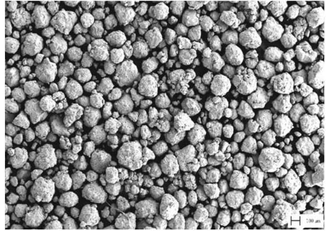
Fig. 11—Structure of powder \text{Cu}_{50}\text{Ti}_{50} after 9 h of mechanical alloying, SEM images at 100 magnifications
