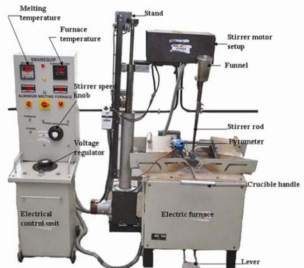
Fig. 2—The experimental set-up used in fabrication of AMMCs (Al 7075- SiC-B 4 C)
