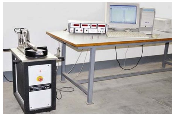
Fig. 6—Pin-on-disc sliding wear testing machine with integrated system
