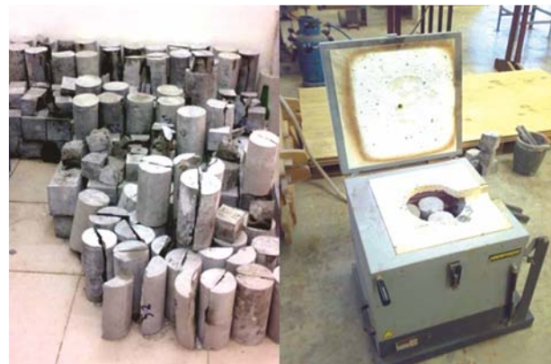
Fig. 1—Concrete samples and electric heating furnace used
