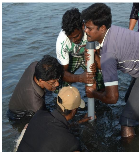
Fig 2. Core sample collection using PVC pipes
