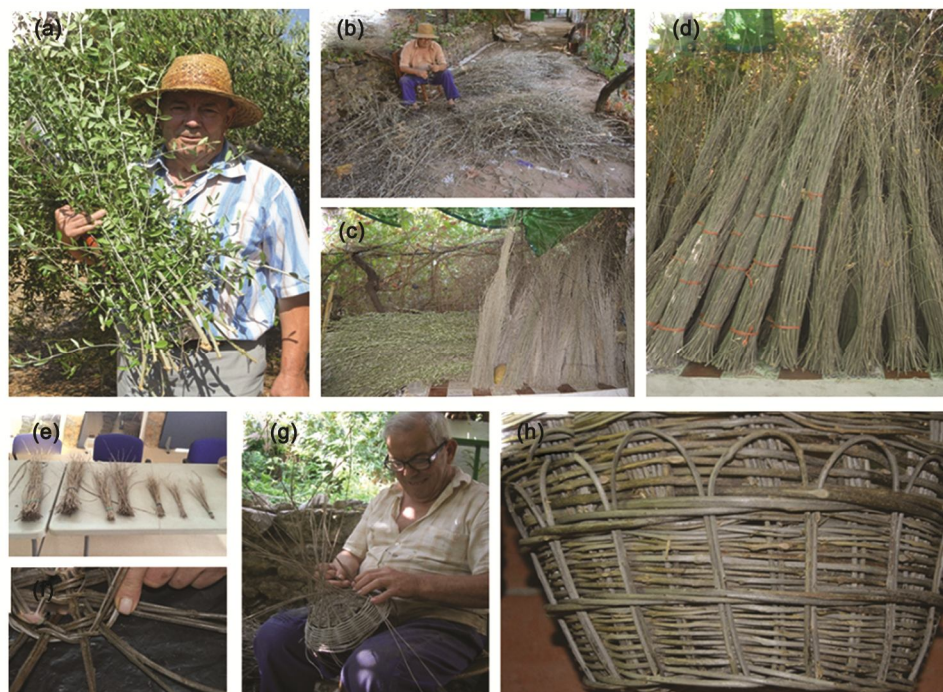
Fig. 3 — Rod selection; (3a&b)—Sucker branches collected and cleared of knots; (3c)—Drying rods; (3d)—Classification by thickness; (3e)—Raw material for manufacturing; (3f)—Doming rods to twist a center; (3g)—Basket manufacturing; (3h)—Filling weft.
