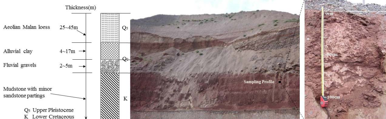
Fig. 1 — Lithological stratigraphic sequence and paleo-weathering profile of Cretaceous red-bed mudstone
