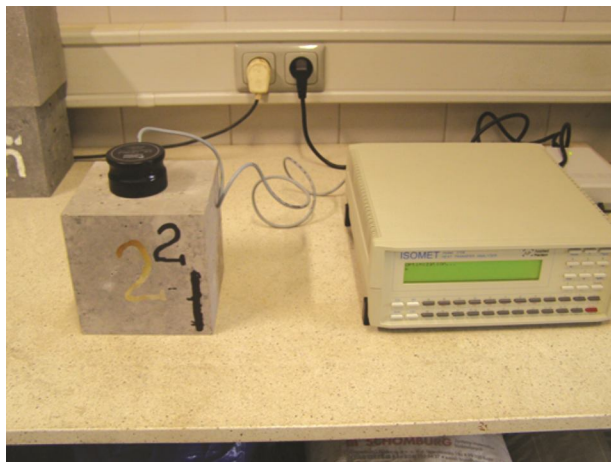
Fig. 3 — Thermal conductivity coefficient measurement using an Isomet device
