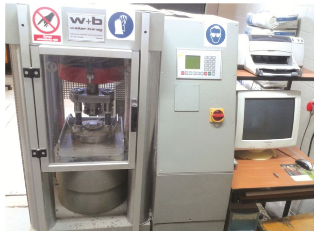
Fig. 2 — Compressive strength test using a Walter+baia 107/3000A/J press
