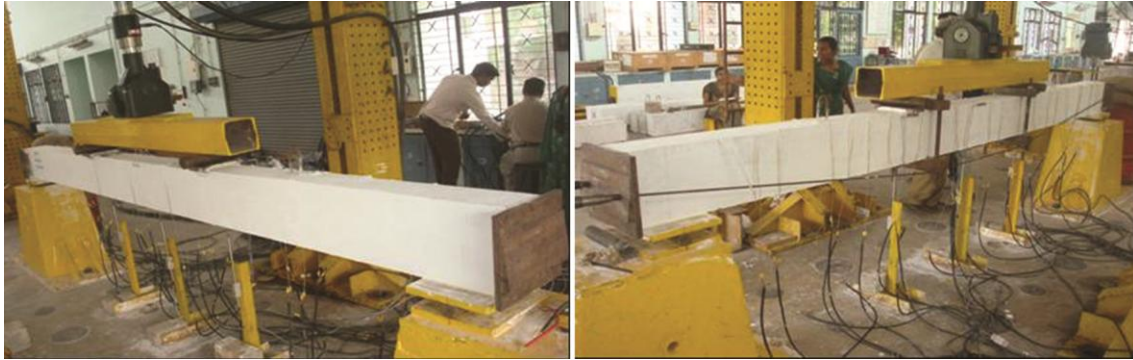
Fig.1 — Test setup and testing of distressed RC specimen retrofitted by external Prestressing EPS-B7
