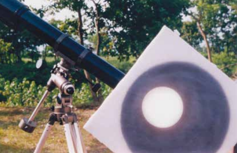
Telescope eyepiece projection system (Back Projection) projecting Sun during Transit of Venus in 2004. The white circle is Sun and small black dot at 6 hr position is Venus
