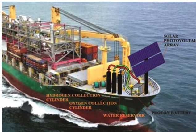
Fig. 1 — A typical marine ship equipped with a novel stand-alone proton battery-based power supply system
