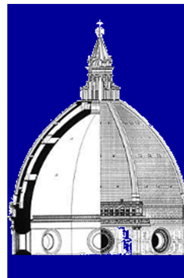
The inner structure of the Brunelleschi dome of Florence
