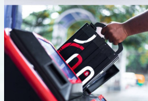
The battery of the Bounce e-scooter can be swapped when discharged
