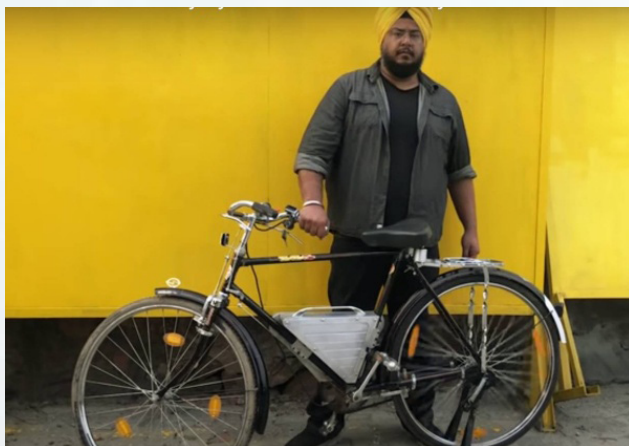
Gursaurabh Singh with a bicycle he retrofitted to work as an e-bike
