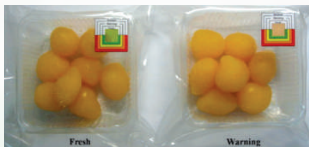
A sensor that monitors carbon dioxide as indication for the freshness of the food item (Credit: https://edepot.wur.nl/298571 )
